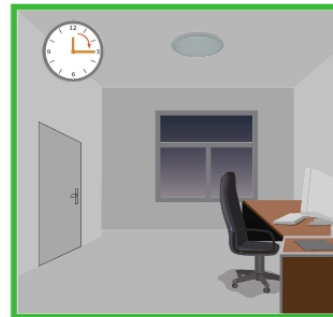
After the dimming delay time, if no one into the sensor area, the lights automatically shut down.
