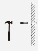
5. Use a hammer to drive the nylon expansion tube into the drilled hole on the wall.
