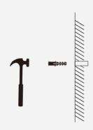
2. Use a hammer to drive the nylon expansion tube into the drilled hole on the wall.
